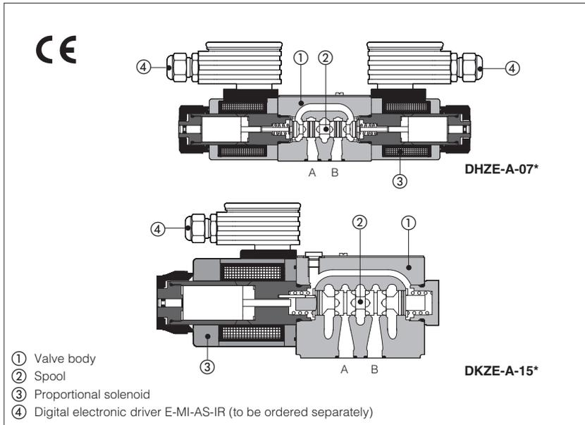
DHZE-A and DKZE-A are open-loop direct operated proportional valves with threaded type proportional solenoids, providing both directional and non-compensated flow control.
