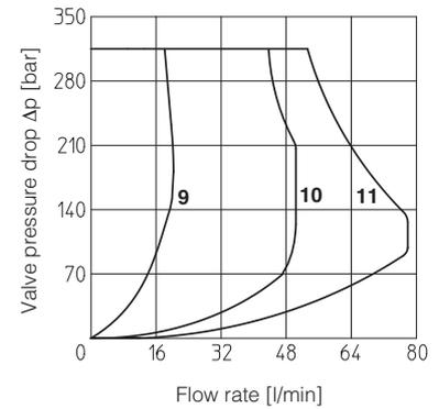
**8 DIAGRAMS FOR DKZE** (based on mineral oil ISO VG 46 at 50 °C)
