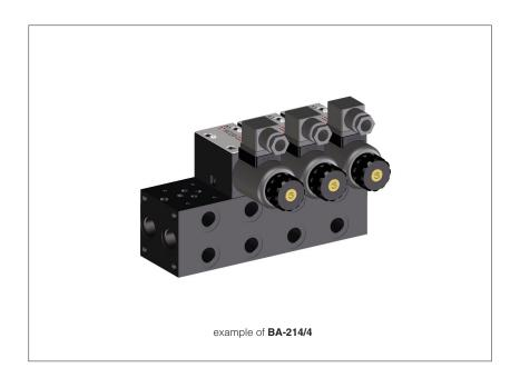
BA-214 and BA-314 are multistation subplates for assembling of directional and modular valves with mounting surface ISO 4401, size 06 and 10.
